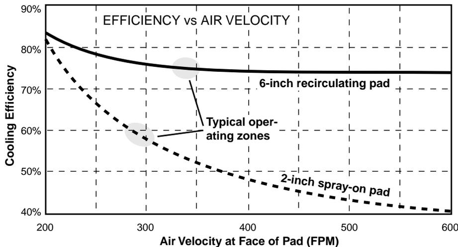
Choosing a cooling pad system involves trade-offs of cooling efficiency, static pressure, and required pad area. As air velocity through a cooling pad goes up, efficiency goes down and static pressure drop increases. To get lower air velocity, for higher efficiency and low static pressure, more pad area is needed. Total house static pressure drop should be kept below 0.10 inches.
