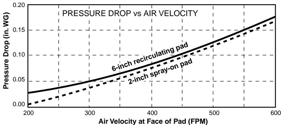
Six-inch small-flute high-efficiency recirculating pad systems typically achieve above 70% cooling efficiency and acceptable house static pressures with design air velocities between 335-350 fpm. To get close to comparable efficiency with a 2-inch spray-on system, air velocity must be lower, typically 280 fpm or slower.
