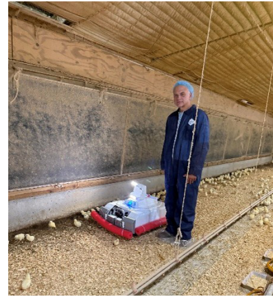
Figure 7. Alabama Extension Specialist Bill Dozier demonstrates an Avirobot inside a broiler house.
