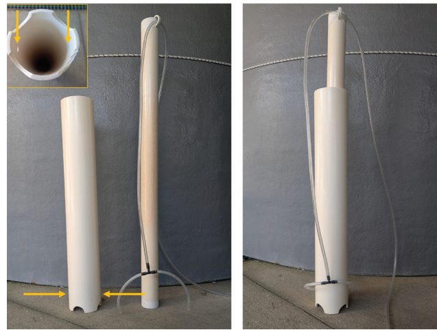
Figure 5. Airlift setup for oyster larval tanks. The left image shows each system component, including a 4-inch PVC airlift pipe with a scalloped bottom edge, a 2-inch center PVC standpipe, and vinyl tubing with U-shaped component. The inset highlights the scalloped bottom edge of the airlift pipe. Yellow arrows indicate the locations of small holes for fitting the tubing. The right image shows the assembled airlift.
