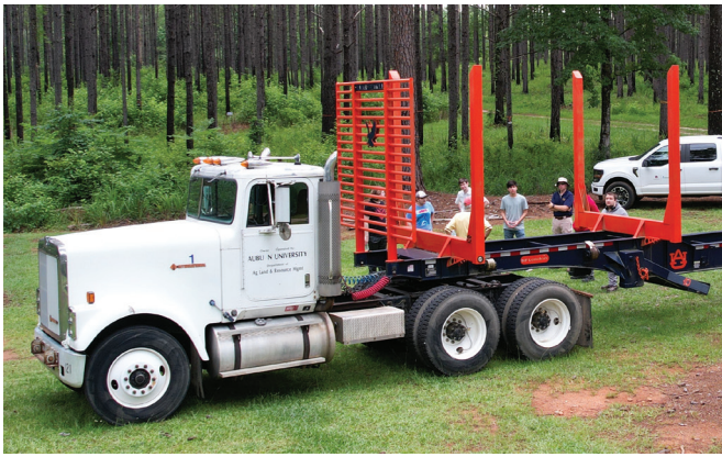
Figure 2. Auburn University log truck and trailer demonstration on transportation challenges and safety in Alabama. Weight and safety inspections, fuel costs, limited turn radius and maneuverability, braking distances, and axle weight and gross vehicle weight limits are some of the challenges.
