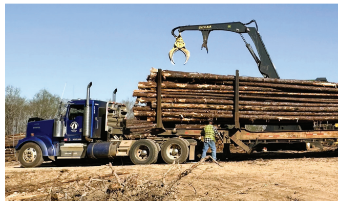
Figure 1. Log truck driver binding a load to get it ready for travel to the mill. This process secures logs with chains, wire ropes, or straps to prevent them from shifting, tipping, or falling off the trailer during transport.
