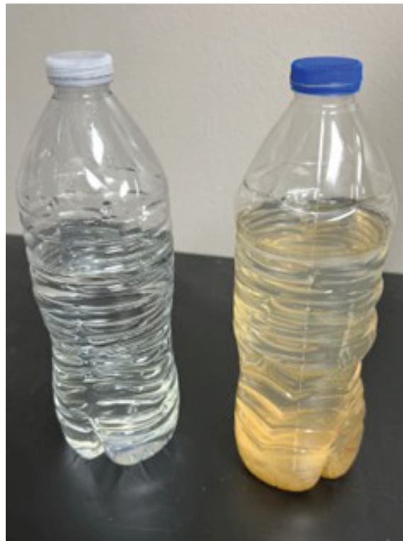
Figure 12. The same water sample as above, re-agitated and treated with alum; picture taken 3 hours after treatment.
