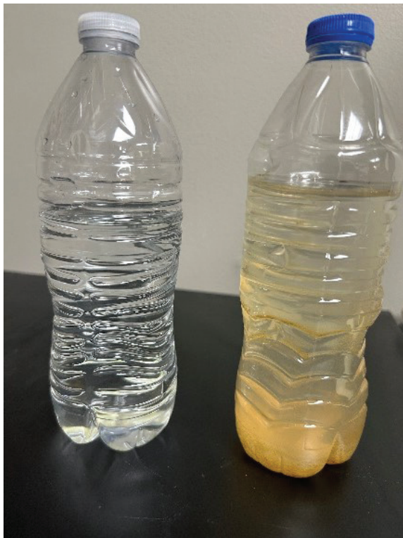
Figure 11. The same water sample as above, re-agitated and treated with alum; picture taken 1 hour and 30 minutes after treatment.
