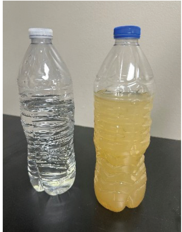
Figure 10. The same water sample as the photo series, re-agitated and treated with alum. This picture was taken zero minutes after treatment.
