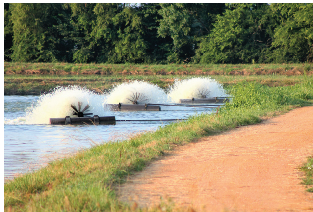
Figure 3. Paddle wheel aerator at a catfish farm in Greene County, Alabama.
