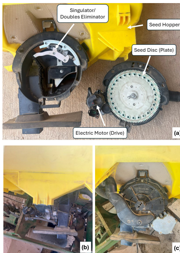
Figure 2. (a) Example of an electric-drive seed meter (Precision Planting vDrive and vSet) and its internal metering components; (b and c) front and back views of the same electric seed meter installed on a seed hopper.
