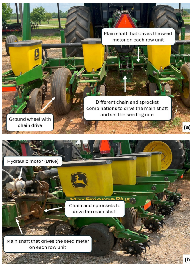
Figure 1. Examples of (a) a traditional ground drive and (b) a hydraulic drive and other main components used for driving seed meters on row crop planters.
