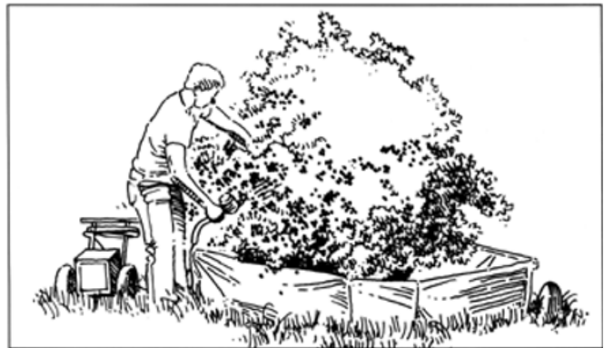
Figure 7. Catch frame and electric vibrator: harvest aid for blueberries
