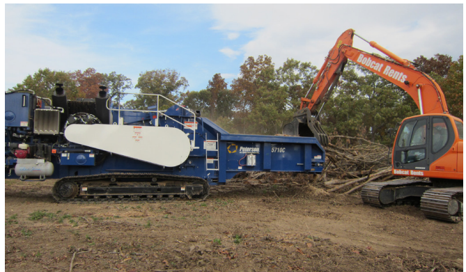
Figure 4. Peterson 5710C whole-tree drum chipper.
