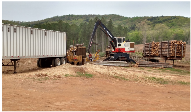
Figure 2. Knuckle-boom loader processing trees and loading woody biomass into an in-woods chipper.
