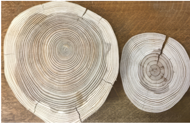
Figure 3. Woody disks sampled from an urban Honey locust ( Gleditsia triacanthos ) tree were destructively sampled (the left disk was derived from the main stem, and the right disk was derived from a large branch). These disks were oven dried, and their dry weight was measured.
