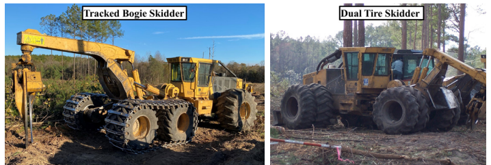
Figure 13. Tracked (left) or dual tire (right) skidders reduce ground pressure and can help minimize soil rutting and compaction when harvesting on wet sites.
