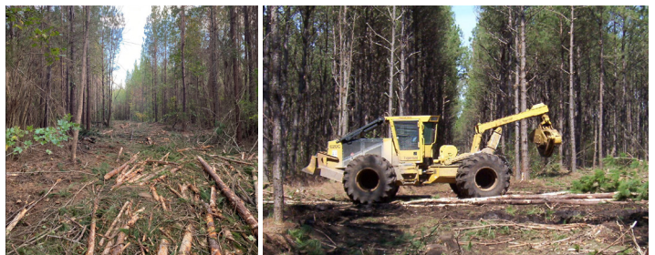
Figure 6. Skidder operator placed slash from the log landing/deck on the main skid trail to avoid soil rutting and compaction while harvesting during wet weather.
