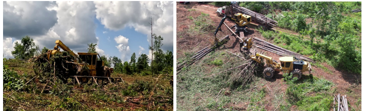
Figure 5. Skidder taking slash from a gate delimer (left) and log landing/deck (right) and spreading it back across the site. This slash can be spread on skid trails for the skidder to drive over to minimize soil rutting and compaction like that seen in figures 3 and 4.
