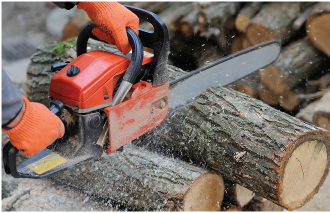
Figure 25. Hold the saw slightly to one side. If you can see into your saw kerf, a kickback can strike your chest or face.
