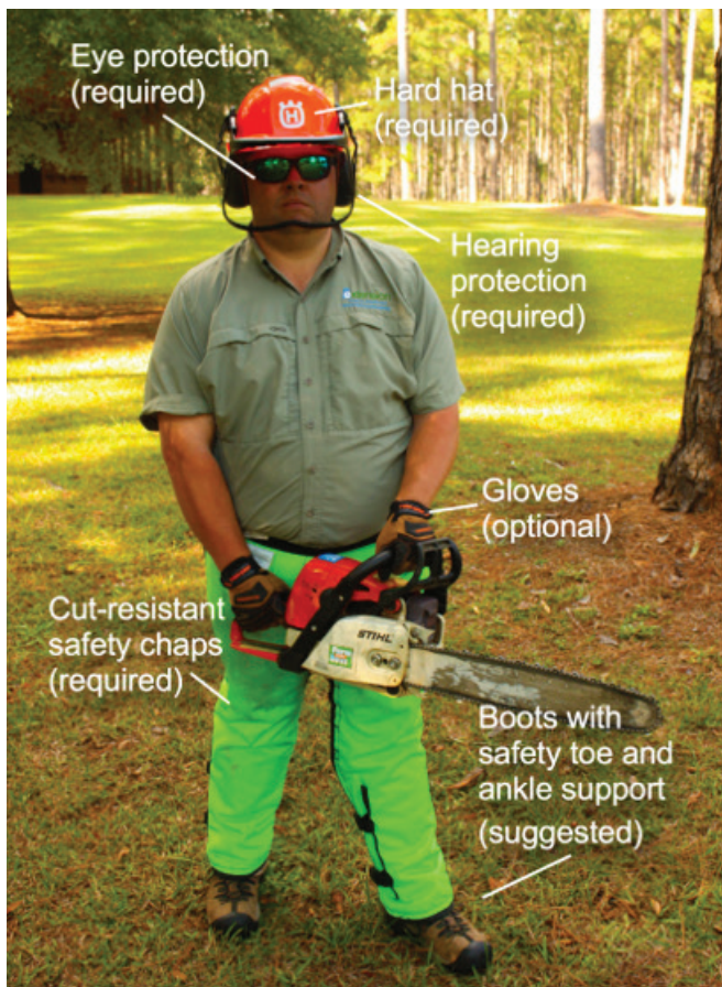
Figure 13. Regardless of whether you run a saw for 5 minutes or 5 hours, wear all your PPE.
