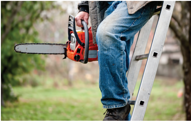
Figure 21. Do not operate saws from a ladder, on roofs, or on top of trees. These are unstable platforms that can shift and move when trees are cut.
