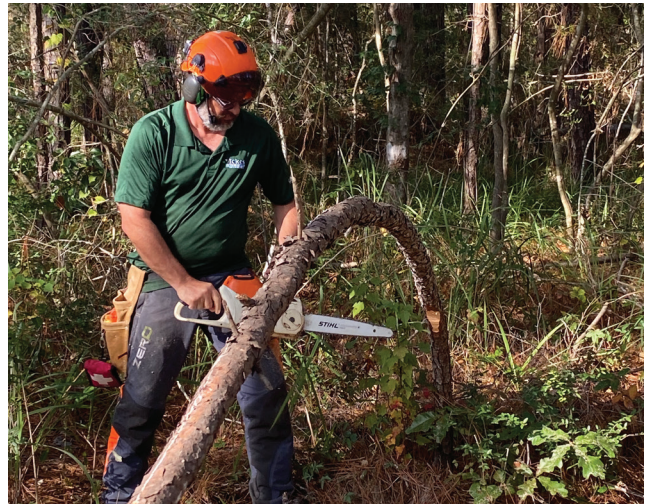
Figure 17. Approach spring poles with extreme caution. If improperly cut, they can result in serious injury.
