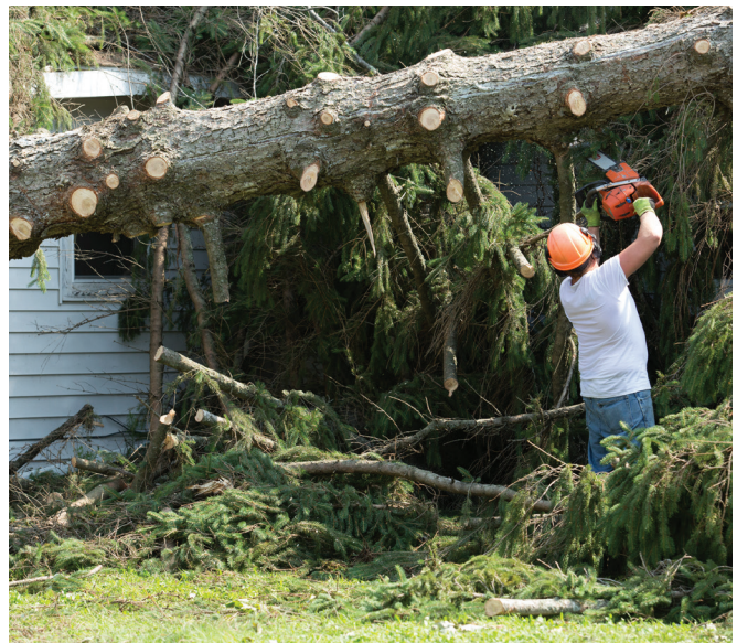
Figure 19. Never operate a saw over shoulder height. You have less control, are more prone to kickbacks, and will physically tire faster.
