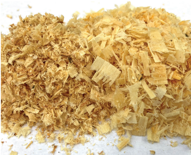
Figure 11. Fine sawdust or increasingly smaller chips are signs of a dull chain, as seen on the left side of the photo.
