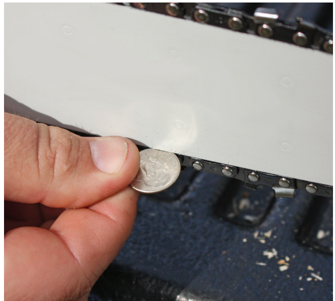
Figure 12. The chain should be tensioned to a dime’s width.
