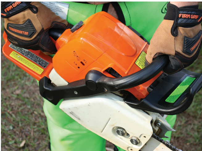
Figure 18. Always use two hands on the saw. Wrap thumbs around handles and engage the chain brake if removing a hand or taking more than two steps.
