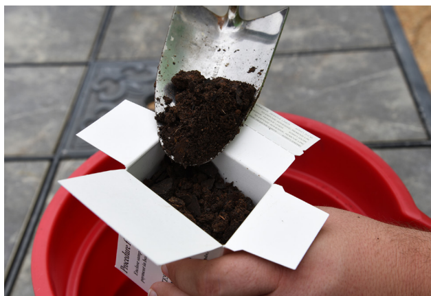
Figure 4. Place about 1 pint of the mixture into a soil sample box.
