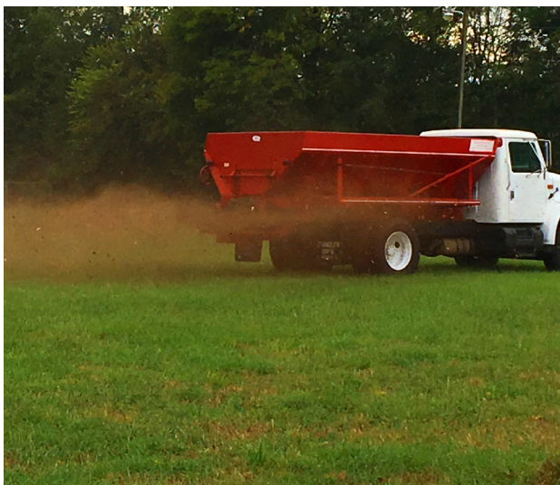
Figure 4. Calibrating the poultry litter applicator before spreading the litter on land.
