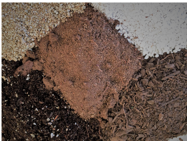
Figure 1. Components of a commercial potting mix. Vermiculite (upper right), perlite (upper left), peat moss (center), pine bark (lower right), and blended components (bottom left).
