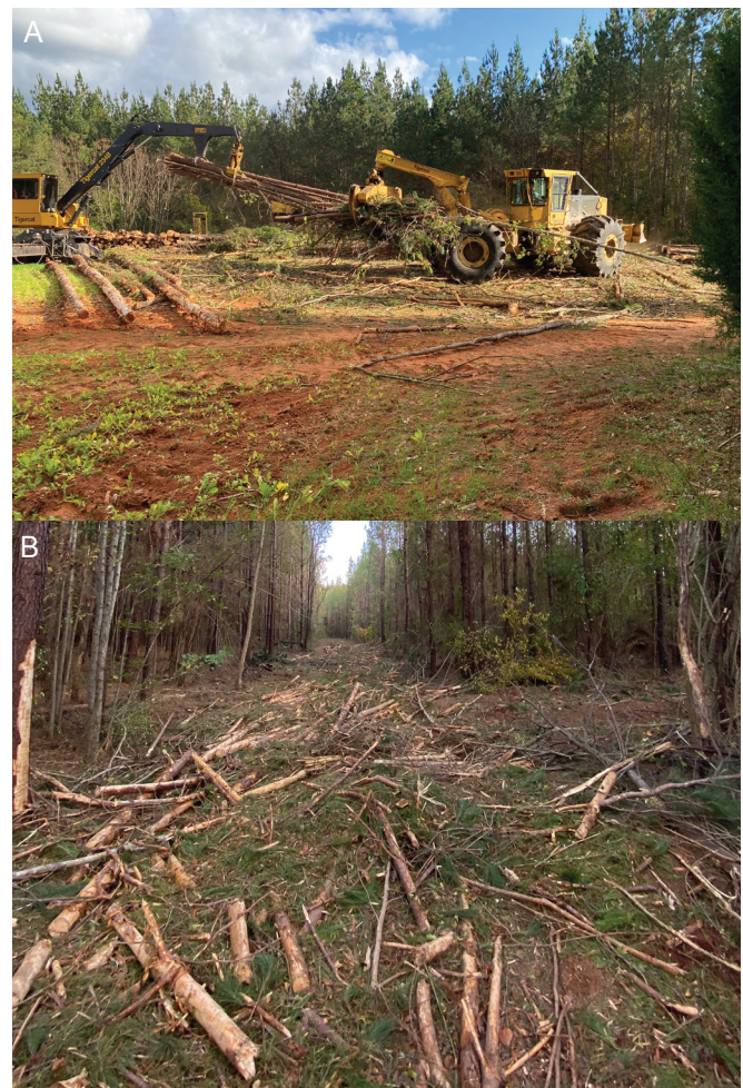
Figure 3. (A) Skidder taking logging slash from the logging deck to spread on high trafficked and erosion susceptible areas and (B) a high trafficked and erosion susceptible area.
