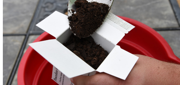
Figure 46. Use a soil sample box to submit to the Soil Testing Lab.
