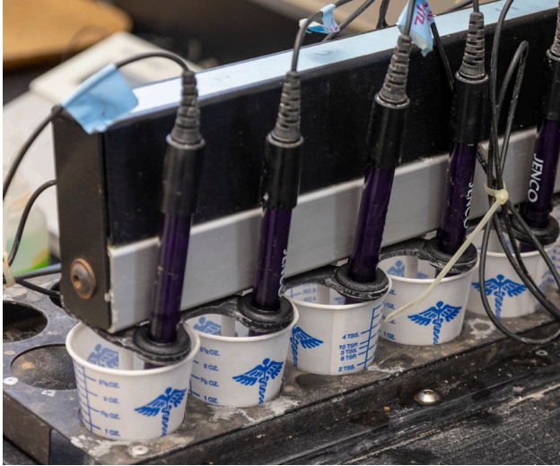
Figure 44. Soil samples are processed to determine soil pH, soil buffer pH, and plant-available nutrient content.
