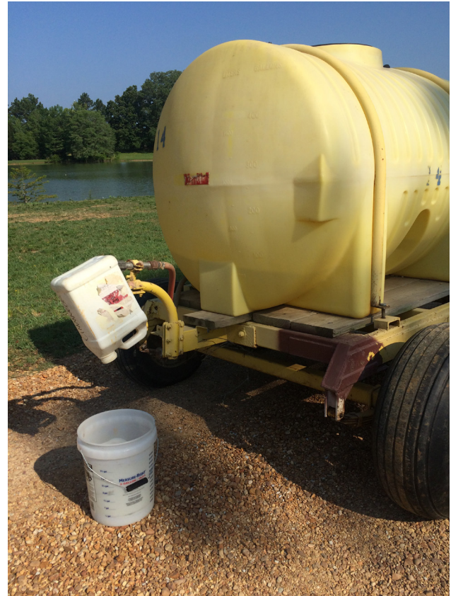
Figure 76. Using a clean container fitted over a boomless nozzle works well as a funnel to determine sprayer output.
