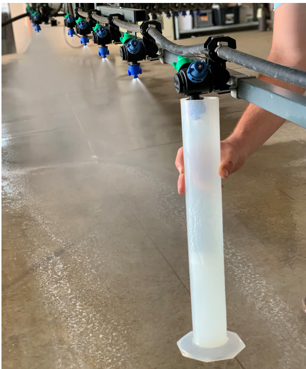
Figure 75. Calibrating a boom sprayer requires catching output from individual nozzles in fluid ounces for the calculated time.
