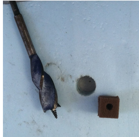
Figure 9. Auger drill bit used to drill holes for cubed media
