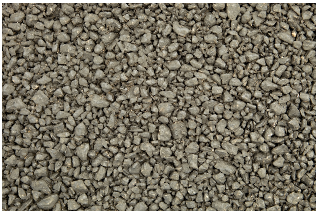
Figure 6. Example of pervious asphalt. The larger aggregate and lack of sand create voids that allow water to flow through the surface rather than run off.
