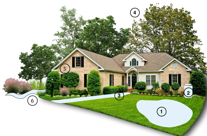
Figure 1. Rainscaping helps prevent polluted runoff from reaching local water bodies. (1) Rain gardens can help capture stormwater runoff, (2) rain barrels can help store water for later release into the landscape, (3) permeable pavement can help water infiltrate into the ground, (4) trees and vegetation help reduce runoff, (5) turf management and turf planting alternatives reduce runoff, and (6) vegetated buffers along streams provide for wildlife habitat and protect the stream bank.
