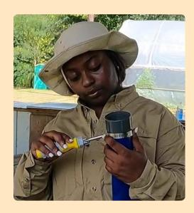
**Step 1.** Begin by using a clamp to attach a gray barbed connector to a lay flat header. If it is hard to get on, use food grade lubricant such as vegetable oil. Tighten the clamp.
