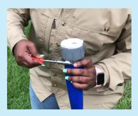
**Step 4.** Push the clamp to the top of the fitting. Use a flathead screwdriver to tighten the clamp.
