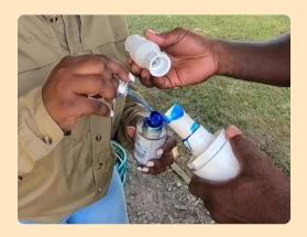
**Step 6.** Apply more PVC glue to attach the backflow preventer or check valve to the PVC. The valve must allow flow in the correct direction, so double-check the direction that the arrow points.
