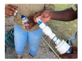
**Step 7.** Apply PVC glue to attach another short piece of PVC pipe and then a <sup>3</sup>/<sub>4</sub>-inch female connector.
