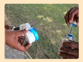
Step 3. Apply PVC glue to the outside of the 34-inch female reducer threading and the inside of the 2-inch male PVC couplet.
