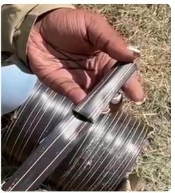
**Step 5.** Fold the tape over twice and then in half so it will easily slip inside the cutoff piece.
