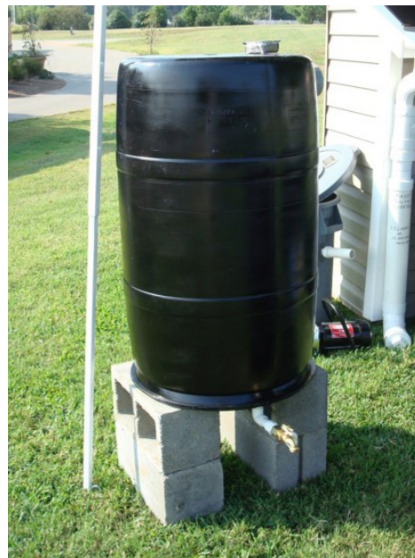
Figure 7. Rain barrel made out of recycled syrup barrel, placed upside down with a PVC connector
