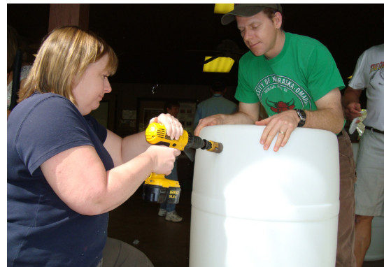
Figure 35. Drilling spigot hole in rain barrel
