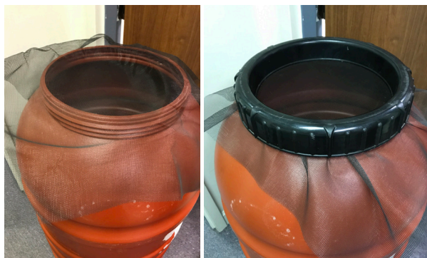
Figure 31. Fiberglass window screen for reused olive barrel
