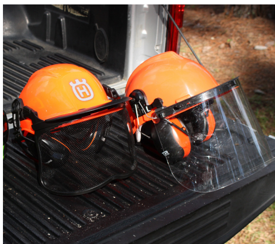
Figure 8. Hard hat face shields can be clear plastic or mesh.
