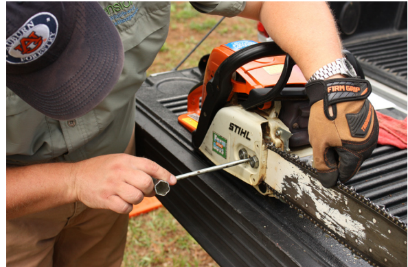
Figure 11. Gloves should be worn when performing saw maintenance.
