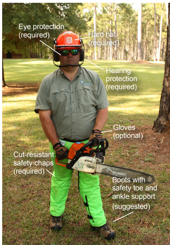
Figure 1. Personal protective equipment (PPE) that should be used when operating a chainsaw.
