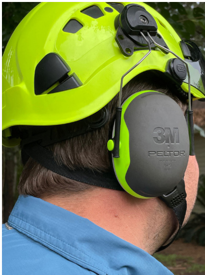
Figure 10. Ear muffs should fit snugly over the entire ear.
