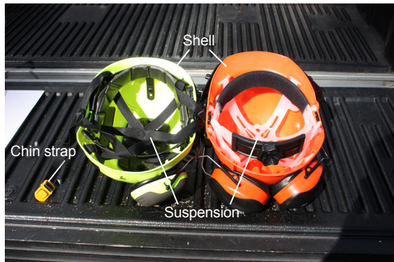
Figure 3. Essential components of a hard hat.
