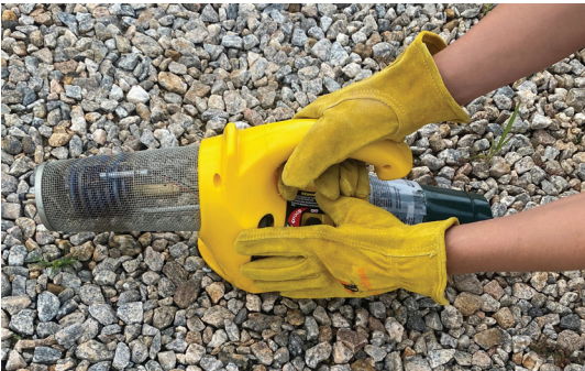
Figure 8. Turn the ignition knob to the open position and push the auto-ignite button until the fogger lights. Keep all body parts and flammable material away from the mesh burner.
