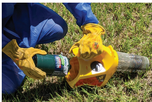
Figure 6. Turn the ignition knob (top) to the off position and connect the propane tank to the fogger (bottom).
