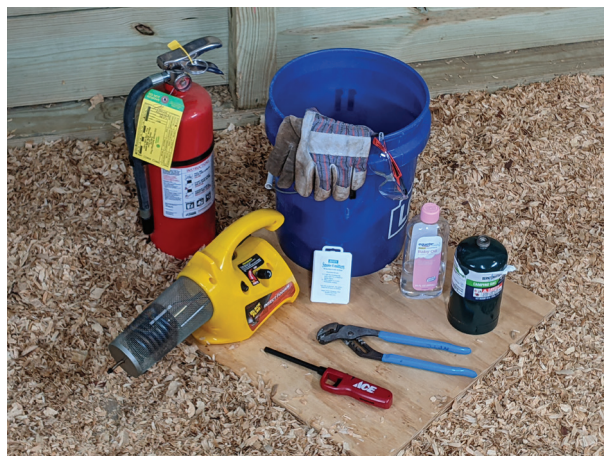
Figure 1. Tools to perform a smoke test: insect fogger, lighter, channel locks, smoke emitters, oil, propane cylinder, safety glasses, leather gloves, fire extinguisher, and bucket of dirt or sand.
