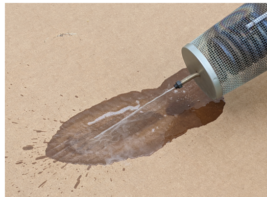
Figure 11. Oil dripping from the nozzle means you may need to let the fogger preheat longer or you may need to slow down your pumping speed. Cardboard in this figure is for illustration purposes only. Make sure you light the fogger on the ground away from flammable materials.
