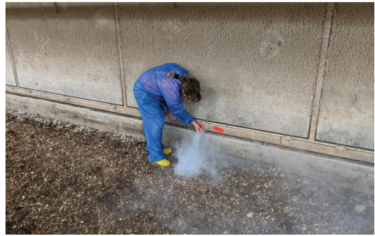
Figure 13. Mark all locations where smoke enters the house perimeter with something bright and easy to see: marking tape, spray paint, etc. Here we are using red tape to identify a large leak at the base of the tunnel door.
