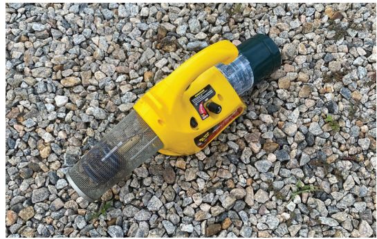
Figure 9. Let the fogger preheat on the ground or other nonflammable surface and away from flammable materials until the fogger produces good fog quality when the trigger is pulled.
