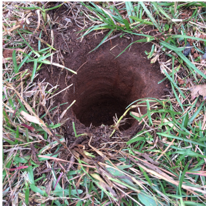
Figures 16. Digging a hole 1 foot deep to conduct an infiltration test.
