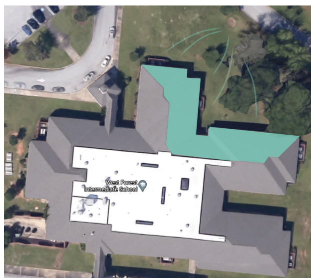
Figure 21. Image highlighting the portion of the rooftop that will drain to the rain garden site. The estimated square footage of this portion of the roof is 7,881 square feet.
