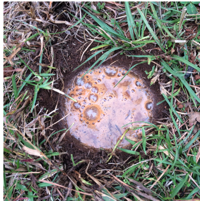
Figures 17. Filling the hole with water to determine infiltration rate.
