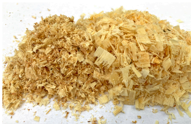
Figure 7. Wood components from a dull chain will be a fine sawdust (left). A sharp chain will have wood shavings (right).
