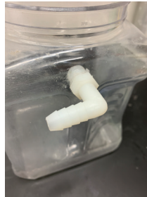
Figure 8. Nylon barbed elbow inserted into the hole on the container
