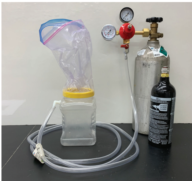
Figure 12. Assembled carbon dioxide euthanasia system
