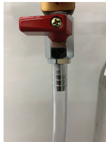
Figure 11. Clear PVC flexible tubing attached to the low-pressure regulator
