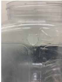
Figure 6. A 3/8-inch hole drilled into the side of the container
