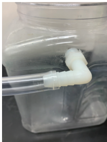
Figure 10. Clear PVC flexible tubing attached to the nylon barbed elbow
