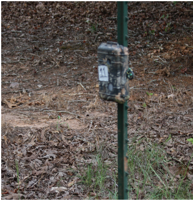
Figure 8. If necessary, use a t-post to correctly position cameras.
