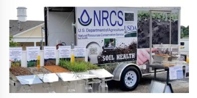
In this demonstration, rainfall is simulated on five different land management systems. The rainfall simulator highlights different methods to reduce soil run off.
