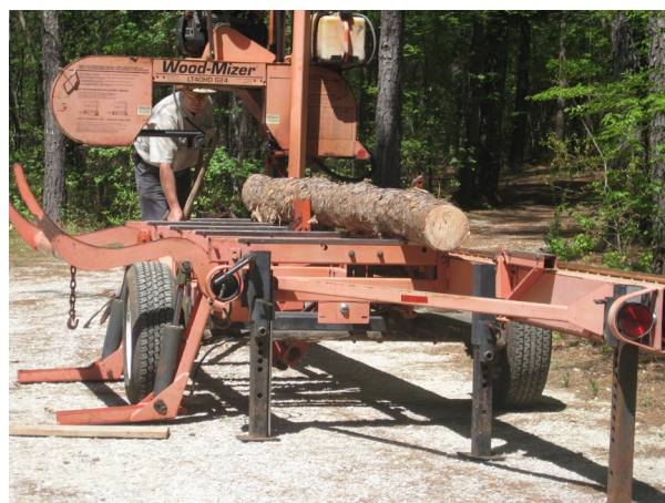
Portable sawmills can be moved to the location where trees will be harvested, eliminating the need to transport logs.
