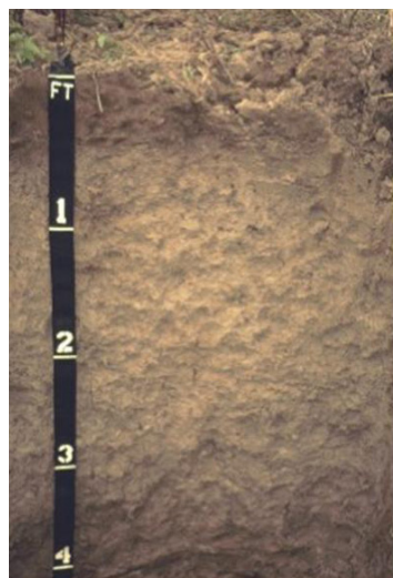
Figure 2. This Houlika silty clay is a deep, somewhat poorly drained, very slowly permeable, acidic soil found in the flood plains of the Black Belt region.
