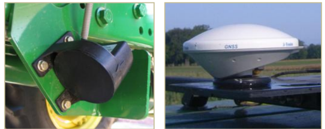
Figure 1. Example ground speed radar mounted on a tractor (left) versus GPS receiver (right) providing simulated ground speed radar output.
