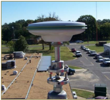
Figure 4. Example CORS station (courtesy of NGS).
