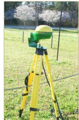
Figure 3. Example RTK base station using a StarFire GPS receiver.
