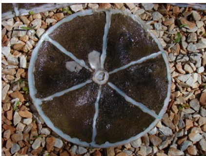
a. Filtered material (100 mesh filter)
