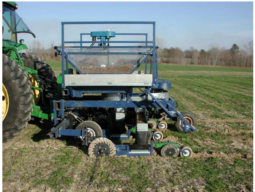
Figure 1. Left side view of the four-row prototype implement for subsurface band application of poultry litter developed at the USDA-ARS National Soil Dynamics Laboratory (Auburn, Alabama).
