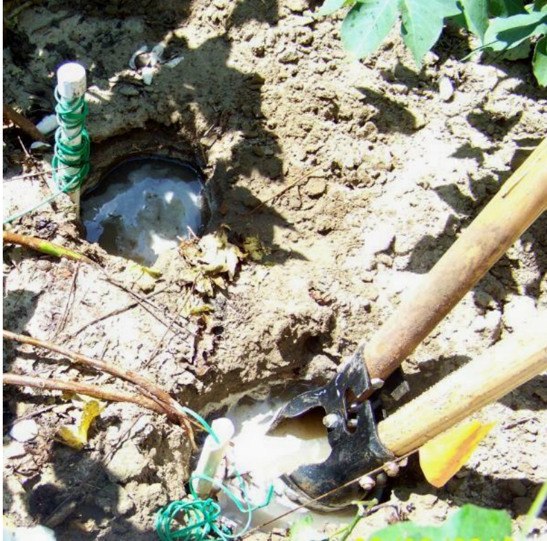
Figure 2 - Soaking hole digger holes with water to soften soil surrounding sensors.
