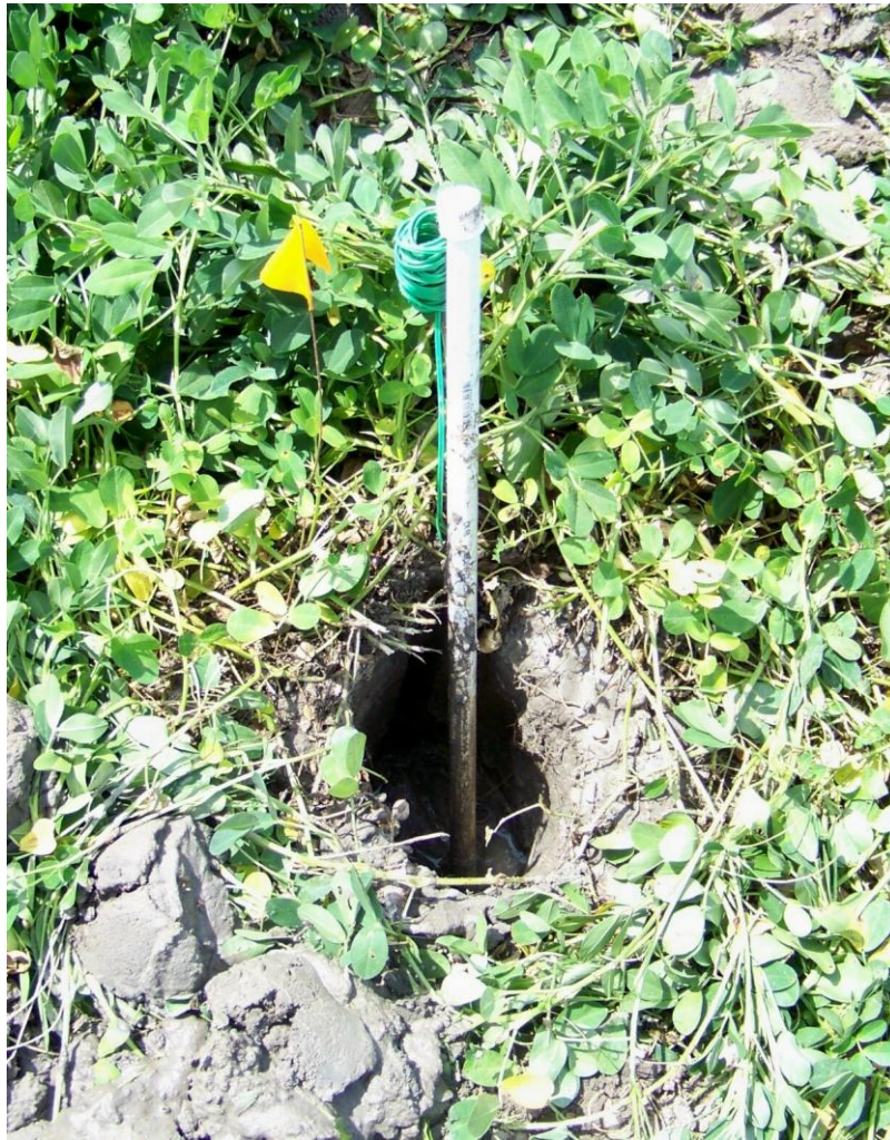
Figure 4 - Soil sensor easily pulled out by hand after water soaking in a peanut field.
