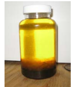
Figure 1. Glycerol (bottom) settling in a sample of Biodiesel.
