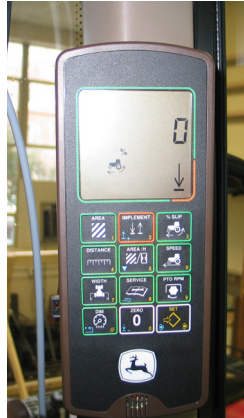
Figure 2. Example performance monitor from a John Deere tractor with the ability to display wheel slip.
