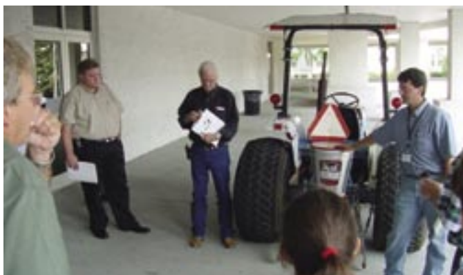
Speaking at a regional imported fire ant workshop last May in Anniston, Regional Extension Agent Chip East demonstrates how a seeder typically used to plant pastureland forages can be modified to apply fire ant bait over large areas.
