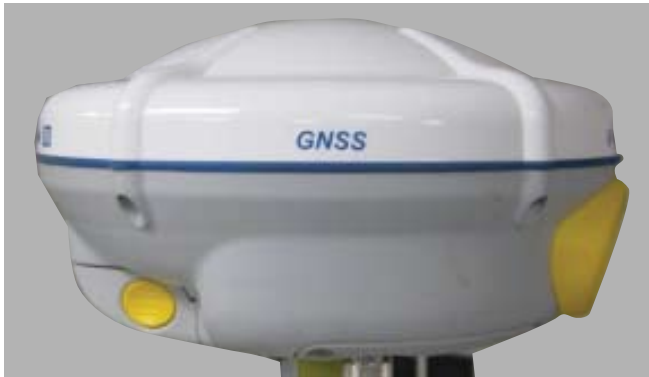
Figure 1. Example GNSS-compatible receiver with “GNSS” labeled on the rim. Most compatible antennas/receivers will carry this label in an easily identifiable location.
