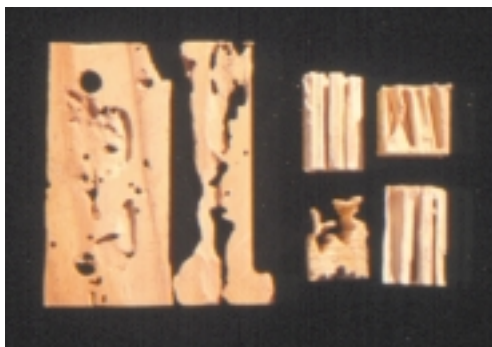
Figure 3. Drywood termite wood damage (left) compared to subterranean termite wood damage (right)
