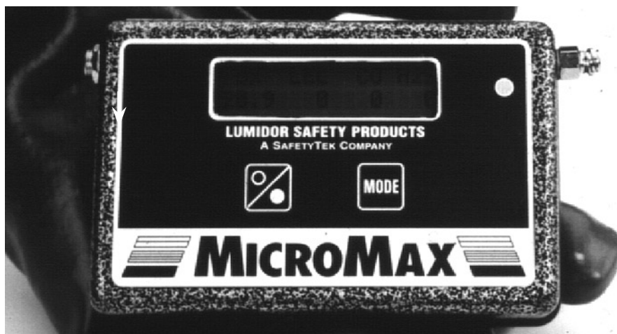
Figure 4. Hand-held, digital, continuous exposure meter used to monitor the concentration of phosphine gas.
