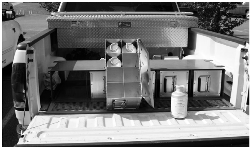
Figure 3. A safe storage box for transporting flasks of aluminum phosphide.
