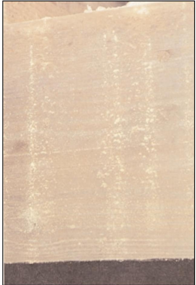
Sometimes powderpost beetle damage creates lines of wood dust on infested lumber.
