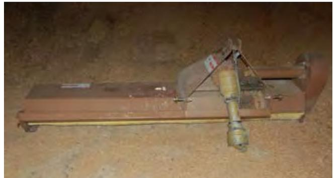
A shallow-tine roto-tiller is an excellent tool for conditioning litter after decaking. Growers should be aware that tilling too deep can contribute to ammonia problems. This shallow tine tiller, which can be pulled behind a 40 hp tractor and do a typical house in less than an hour, is often used to depths of only 1 to 2 inches to mix and condition the surface after decaking.
