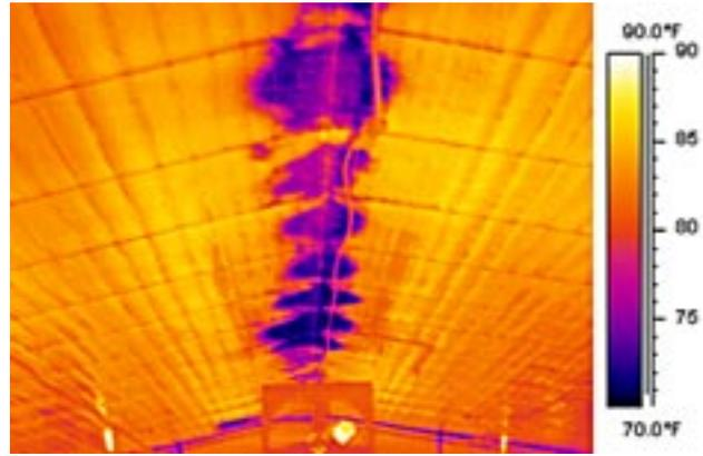
Thermal photos above, taken in two different broiler houses during brooding, show dramatic differences in temperature along the ceiling, with darker areas cooler and lighter areas warmer, caused by blown-in insulation having shifted away from the centerline peak area above the triply. The houses will lose a significant amount of heat through these uninsulated areas, causing increased heating cost and possibly affecting flock performance.
