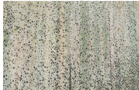
Severe algae growth has almost completely clogged this pad. Don't ever let your pads get this bad!
