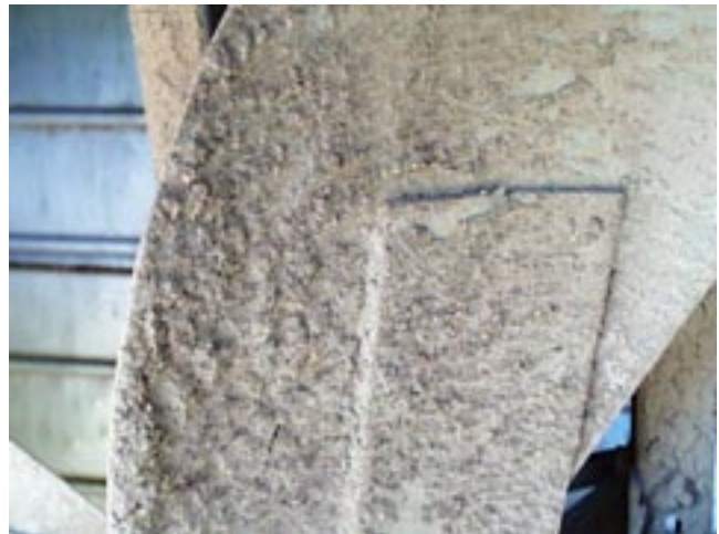
Photo at right is a close-up view of a fan blade that has not been cleaned for several weeks. The dust and dirt build-up changes the aerodynamics of the blade and puts additional drag on the blade, severely reducing fan performance.
