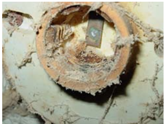
Old keyless sockets, as shown at left above and in close-up at right, are highly susceptible to corrosion in the broiler house, leading to higher bulb failures and dimming problems. For this reason, bulb manufacturers highly recommend using only nickel-plated brass sockets for both CC and CFL bulbs.
