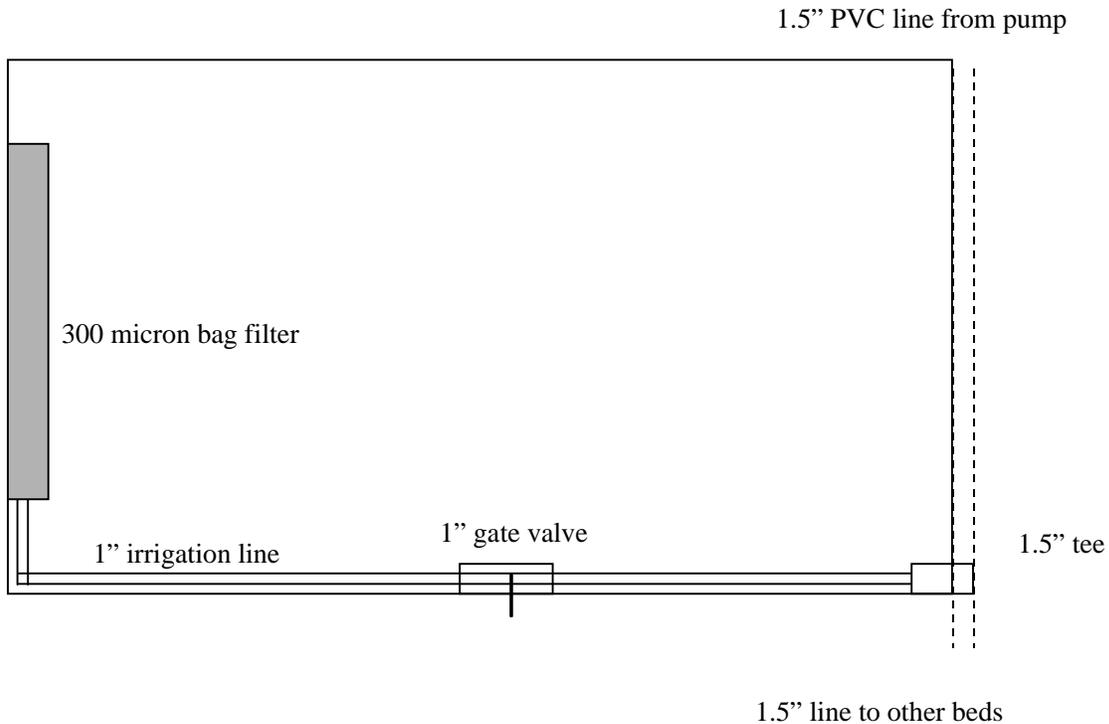
Figure 7 Overview of growing bed irrigation system.
