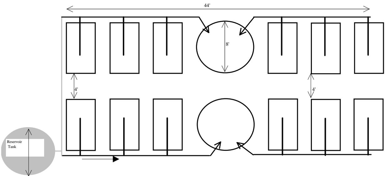
Figure 2 Overview of the return flow lines.
