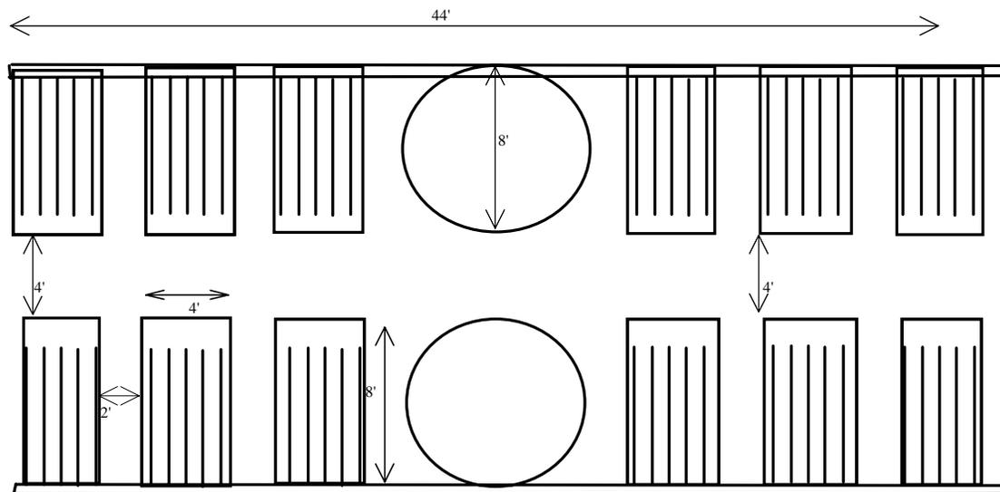
Figure 8 Overview of root zone heating system.
