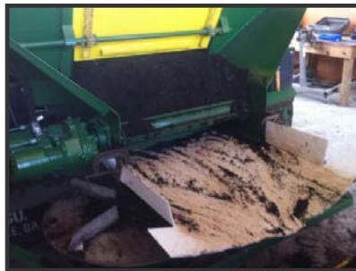
Figure 4. Illustration of the conveyor being full of material and the fabricated chute for directing material into the catch pan.
