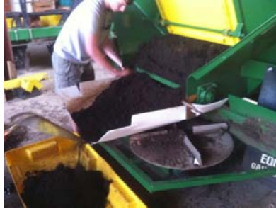
Figure 5. Material flowing from conveyor, onto slide, and into a collection device (e.g. tub).
